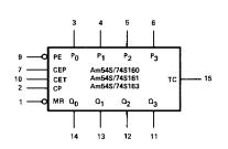
$V_{CC} = Pin 16$ GND = Pin 8
