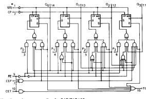
\*MR is asynchronous on the Am54S/74S161 and synchronous on the Am54S/74S163
