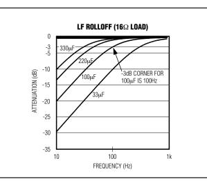
Figure 2. Low-Frequency Attenuation for Common DC-Blocking Capacitor Values
