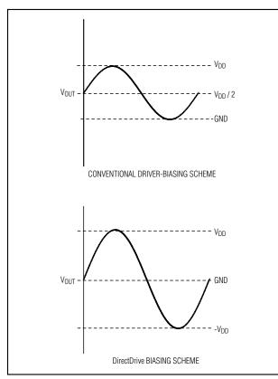
Figure 1. Traditional Driver Output Waveform vs. MAX9721 Output Waveform (Ideal Case)
