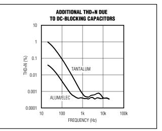
Figure 3. Distortion Contributed By DC-Blocking Capacitors
