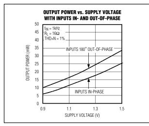
Figure 4. Output Power vs. Supply Voltage with Inputs In-/Outof-Phase
