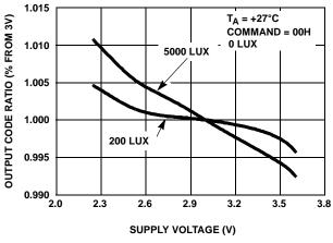
FIGURE 15. OUTPUT CODE vs SUPPLY VOLTAGE
