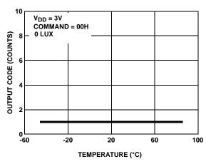
FIGURE 18. OUTPUT CODE FOR 0 LUX vs TEMPERATURE
