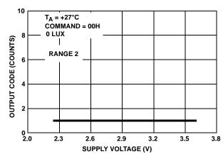
FIGURE 14. OUTPUT CODE FOR 0 LUX vs SUPPLY VOLTAGE
