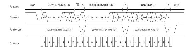
FIGURE 2. I<sup>2</sup>C WRITE TIMING DIAGRAM SAMPLE
