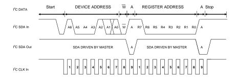
FIGURE 3. I<sup>2</sup>C sync\_iic TIMING DIAGRAM SAMPLE
