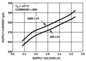
FIGURE 13. SUPPLY CURRENT vs SUPPLY VOLTAGE
