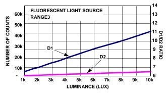
FIGURE 8. D1 AND D2 FLUORESCENT LIGHT SOURCE RESPONSE
