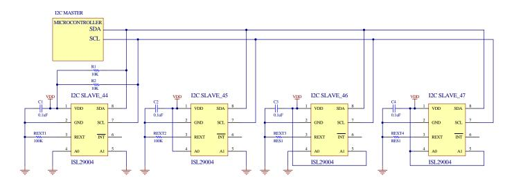
FIGURE 6. ISL29004 TYPICAL CIRCUIT
