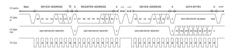
FIGURE 1. I<sup>2</sup>C READ TIMING DIAGRAM SAMPLE
