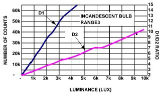
FIGURE 11. D1 AND D2 INCANDESCENT LIGHT SOURCE RESPONSE
