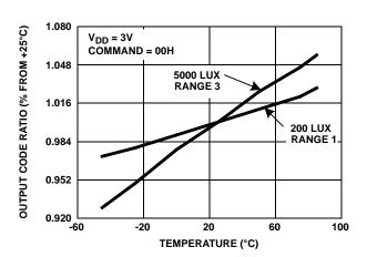
FIGURE 19. OUTPUT CODE vs TEMPERATURE
