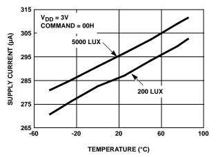
FIGURE 17. SUPPLY CURRENT vs TEMPERATURE
