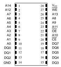
28-Pin Encapsulated Package 740-Mil Extended
