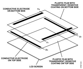
Figure 22. Basic Construction of a Touch Screen
