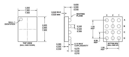
Figure 48. 12-Ball, Backside-Coated Wafer Level Chip Scale Package [WLCSP] (CB-12-5) Dimensions shown in millimeters
