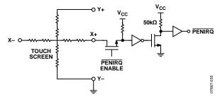
Figure 36. PENIRQ Output Equivalent Circuit
