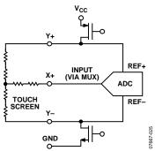
Figure 25. Ratiometric Conversion of Touch Screen Inputs
