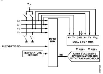
Figure 23. Analog Input Structure
