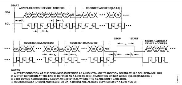
Figure 43. Example of I<sup>2</sup>C Timing for Single Register Write Operation
