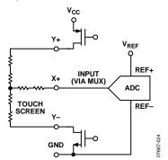
Figure 24. Single-Ended Conversion of Touch Screen Inputs
