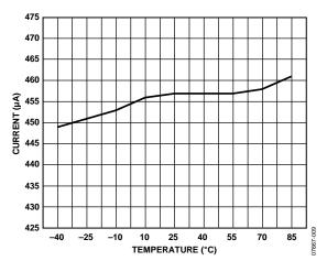
Figure 9. Supply Current vs. Temperature
