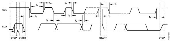
Figure 3. Detailed I<sup>2</sup>C Timing Diagram
