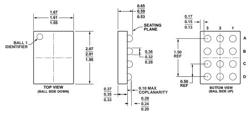
Figure 47. 12-Ball Wafer Level Chip Scale Package [WLCSP] (CB-12-1) Dimensions shown in millimeters
