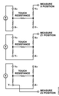
Figure 26. Three Measurements Required for Touch Pressure
