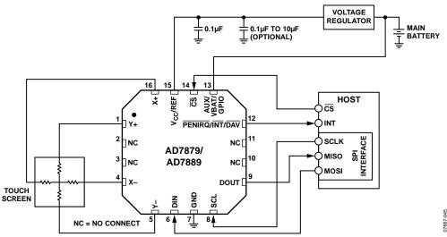
Figure 46. Typical Application Circuit
