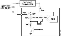
Figure 28. Block Diagram of Battery Measurement Circuit
