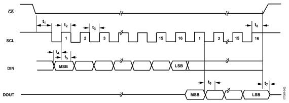
Figure 2. Detailed SPI Timing Diagram
