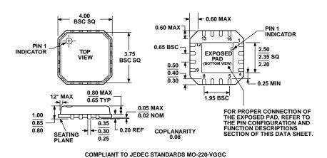
Figure 49. 16-Lead Lead Frame Chip Scale Package [LFCSP\_VQ] 4 mm × 4 mm, Very Thin Quad (CP-16-10) Dimensions shown in millimeters
