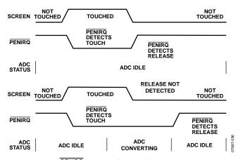
Figure 37. PENIRQ Operation for ADC Idle and ADC Converting
