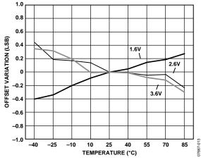
Figure 13. Change in ADC Offset vs. Temperature
