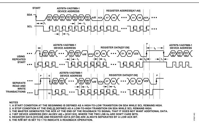
Figure 44. Example of I<sup>2</sup>C Timing for Single Register Readback Operation
