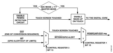
Figure 38. Master Mode Operation
