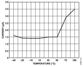
Figure 11. Full Power-Down IDD vs. Temperature
