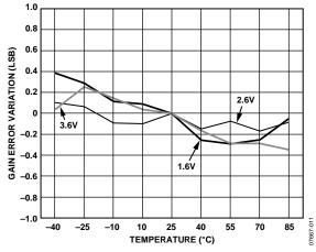
Figure 12. Change in ADC Gain vs. Temperature
