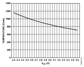
Figure 19. Temperature Code vs.  $V_{CC}$  for 25°C
