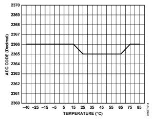
Figure 18. ADC Code vs. Temperature (Fixed Analog Input)
