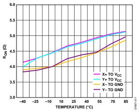
Figure 17. Switch On Resistance vs. Temperature  $(X+, Y+: Pin \text{ to } V_{CC}; X-, Y-: Pin \text{ to } GND)$
