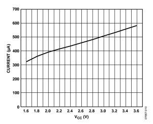
Figure 10. Supply Current vs.  $V_{CC}$
