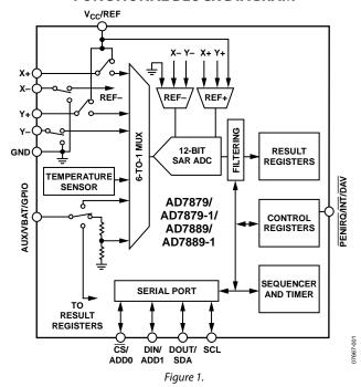
The AD7879/AD7889 have a programmable pin that can operate as an auxiliary input to the ADC, as a battery monitor, or as a GPIO. In addition, a programmable interrupt output can operate in three modes: as a general-purpose interrupt to signal when new data is available (DAV), as an interrupt to indicate when limits are exceeded (INT), or as a pen-down interrupt when the screen is touched (PENIRQ). The AD7879/AD7889 offer temperature measurement and touch-pressure measurement.
