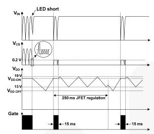
Figure 24. Waveforms in Short-LED Condition
