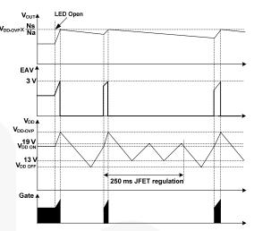
Figure 26. Waveforms in LED Open Condition
