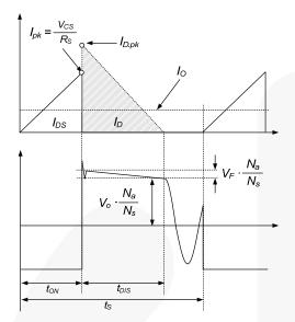
Figure 20. Key Waveforms for Primary-Side Regulation
