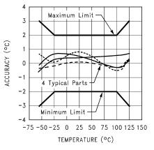
Figure 13. Temperature Accuracy
