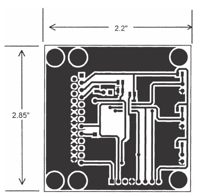
LM75C  $\theta_{JA}$  (thermal resistance, junction-to-ambient) when attached to a printed circuit board with 2 oz. foil similar to the one shown. Summarized below:
