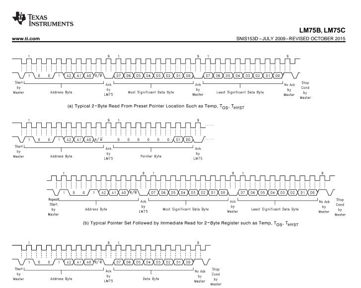
(c) Typical 1-Byte Read From Configuration Register With Preset Pointer
