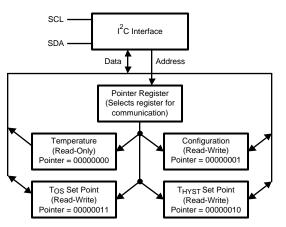
Figure 10. Iternal Register Structure
