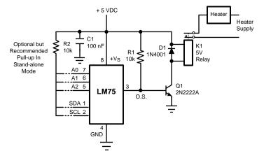
Figure 14. Simple Thermostat, Interface Optional
