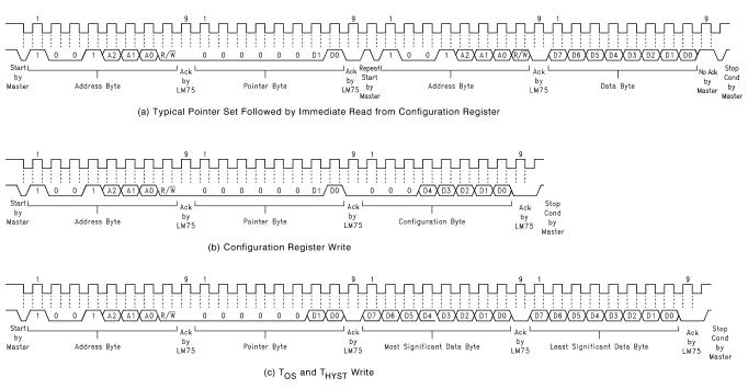
Figure 5. I<sup>2</sup>C Timing Diagrams (Continued)
