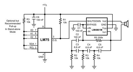
Figure 15. Temperature Sensor with Loudmouth Alarm (Barking Watchdog)
