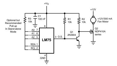
When using the two-wire interface: program O.S. for active high and connect O.S. directly to Q2's gate.
