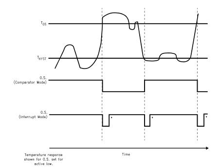
These interrupt mode resets of O.S. occur only when LM75 is read or placed in shutdown. Otherwise, O.S. would remain active indefinitely for any event.
