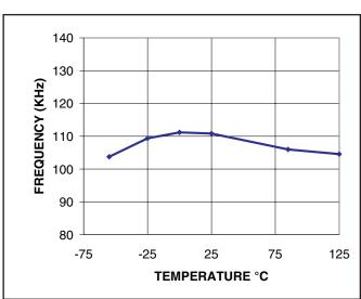
Figure 3. Oscillator Frequency vs. Temperature (CT = 680pF)
