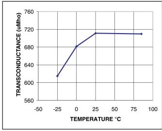
Figure 2. Volt Amp GM (IOUT =  $10\mu$ A)
