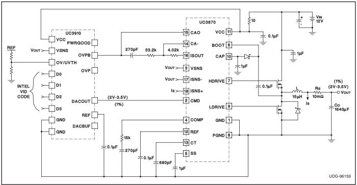
Figure 1. Typical Application: UC3870-1, -2 Pentium Pro Power Converter
