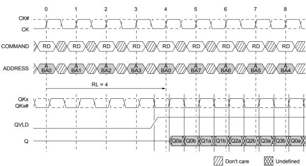
Figure 2-14. READ Burst Basic Sequence: BL=2, RL=4, Configuration 1
