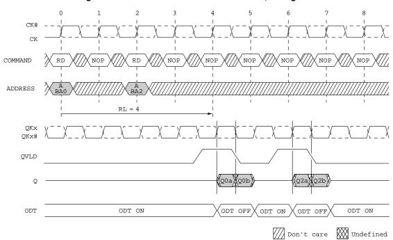
Figure 2-24. READ NOP READ with ODT: BL=2, Configuration 1
