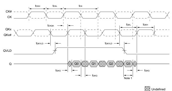
Note Minimum READ data valid window can be expressed as MIN.( $t_{QKH}$ ,  $t_{QKL}$ ) – 2 x MAX.( $t_{QKQx}$ ) tckh and tckl are recommended to have 50% / 50% duty.
