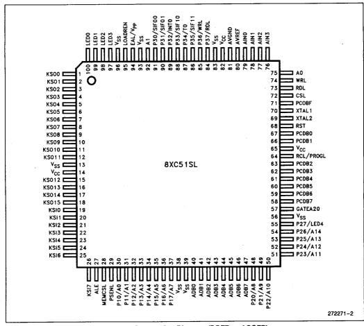
Figure 2. Connection Diagram (PQFP and SQFP)
