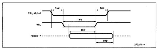
Figure 4. Host-Interface Write
