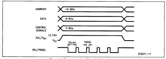
Figure 9. Programming Signal's Waveforms
