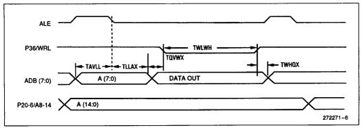
Figure 6. External Data Memory Write
