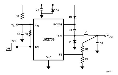
FIGURE 17. LM2738Y (550kHz) V<sub>BOOST</sub> Derived from V<sub>SHUNT</sub> 18V to 1.5V/1.5A
