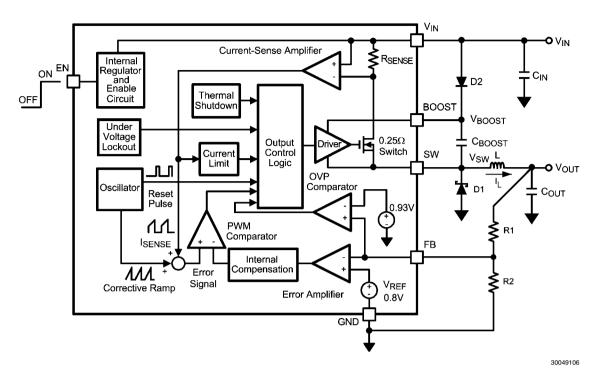
FIGURE 1. Simplified Internal Block Diagram
