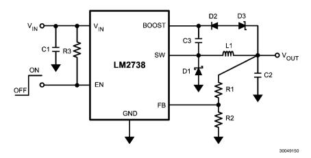
FIGURE 14. LM2738X (1.6MHz)  $V_{BOOST}$  Derived from Series Zener Diode ( $V_{OUT}$ ) 15V to 9V/1.5A
