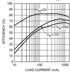
Efficiency vs Load Current - "Y"  $V_{OUT} = 5V$
