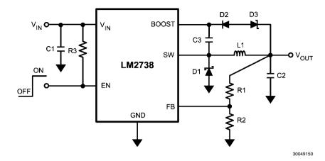
FIGURE 19. LM2738Y (550kHz)
