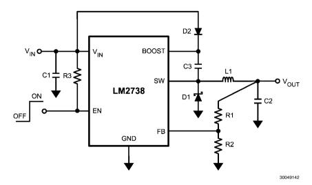
FIGURE 15. LM2738Y (550kHz)
