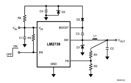
FIGURE 12. LM2738X (1.6MHz) V<sub>BOOST</sub> Derived from V<sub>SHUNT</sub> 18V to 1.5V/1.5A
