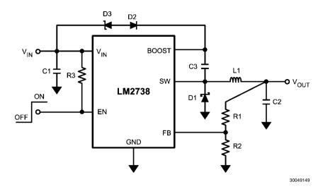
FIGURE 18. LM2738Y (550kHz)  $V_{BOOST}$  Derived from Series Zener Diode ( $V_{IN}$ ) 15V to 1.5V/1.5A
