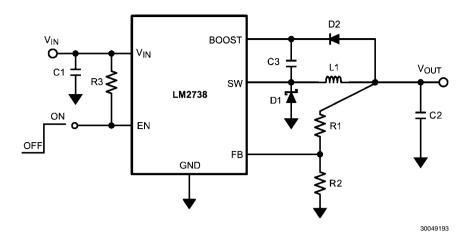
FIGURE 16. LM2738Y (550kHz) V<sub>BOOST</sub> Derived from V<sub>OUT</sub> 12V to 3.3V/1.5A
