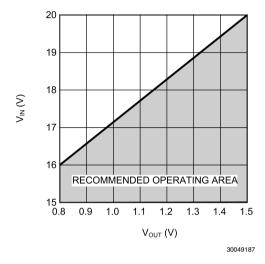
FIGURE 7. LM2738X - 1.6MHz (25°C, LOAD=1.5A)
