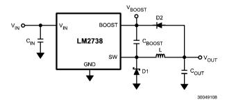
FIGURE 3. V<sub>OUT</sub> Charges C<sub>BOOST</sub>
