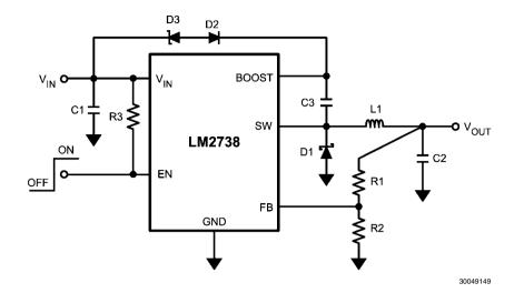
FIGURE 13. LM2738X (1.6MHz)  $V_{BOOST}$  Derived from Series Zener Diode ( $V_{IN}$ ) 15V to 1.5V/1.5A
