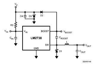
FIGURE 5. Boost Voltage Supplied from the Shunt Zener on  $V_{\rm IN}$
