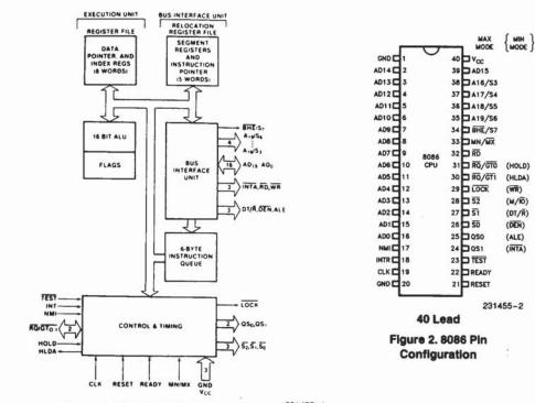
Figure 1. 8086 CPU Block Diagram
