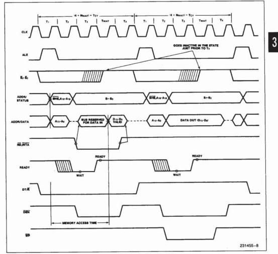
Figure 5. Basic System Timing
