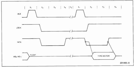
Figure 6. Interrupt Acknowledge Sequence
