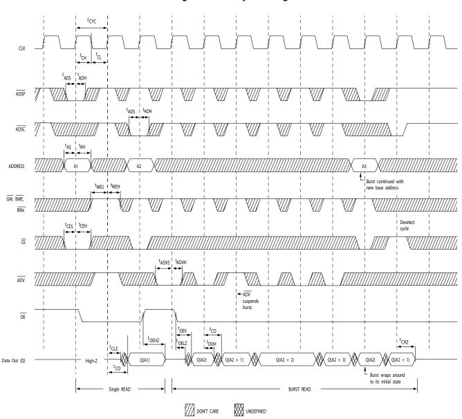
Note 18. On this diagram, when  $\overline{\text{CE}}$  is LOW:  $\overline{\text{CE}}_1$  is LOW,  $\text{CE}_2$  is HIGH, and  $\overline{\text{CE}}_3$  is LOW. When  $\overline{\text{CE}}$  is HIGH:  $\overline{\text{CE}}_1$  is HIGH,  $\text{CE}_2$  is LOW, or  $\overline{\text{CE}}_3$  is HIGH.
