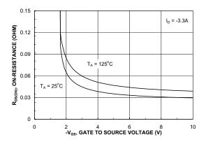
Figure 4. On-Resistance Variation with Gate-to-Source Voltage.
