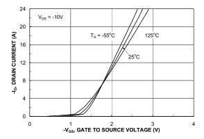
Figure 5. Transfer Characteristics.
