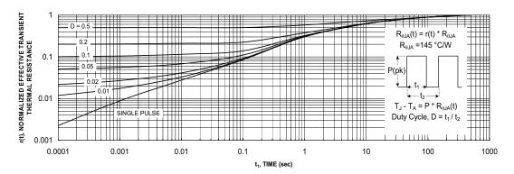
Figure 11. Transient Thermal Response Curve.
