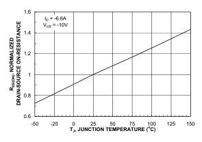
Figure 3. On-Resistance Variation with Temperature.
