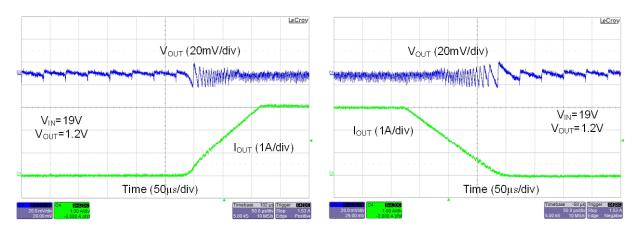
Figure 22. Operation as Load Changes from 0 A to 3 A Figure 23. Operation as Load Changes from 3 A to 0 A
