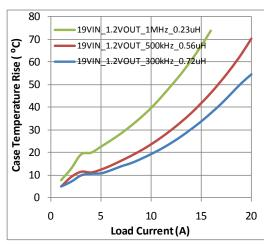
Figure 12. Case Temperature Rise vs. Load Current on Figure 13. Case Temperature Rise vs. Load Current on 4 Layer PCB, 1 oz Copper, 7 cm x 7 cm on 4 Layer PCB, 1 oz Copper, 7 cm x 7 cm
