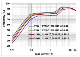
Figure 11. Efficiency vs. Load Current with  $V_{OUT}$ =1.2 V and  $f_{SW}$ =500 kHz
