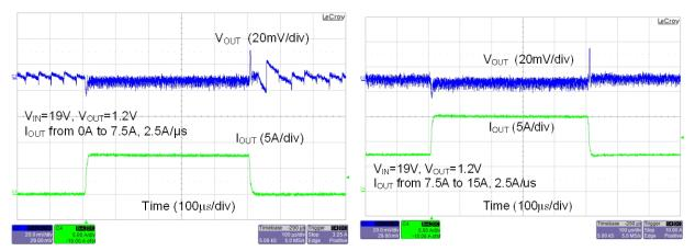
Figure 24. Load Transient from 0% to 50% Load Current
