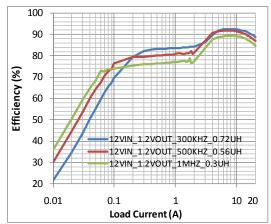
Figure 7. Efficiency vs. Load Current with  $V_{IN}$ =19 V and  $V_{OUT}$ =1.2 V
