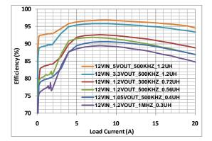
Figure 9. Efficiency vs. Load Current with  $V_{\text{IN}}$ =19 V
