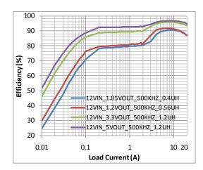
Figure 5. Efficiency vs. Load Current with V<sub>IN</sub>=19 V and f<sub>SW</sub>=500 kHz
