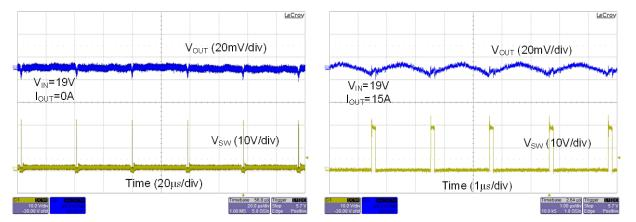
Figure 20. Static Load Ripple at No Load
