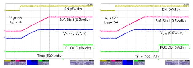
Figure 16. Startup Waveforms with 0 A Load Current Figure 17. Startup Waveforms with 15 A Load Current
