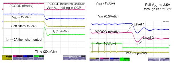
Figure 26. Over-Current Protection with Heavy Load Figure 27. Over-Voltage Protection Level 1 and Level 2
