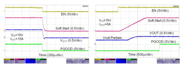
Figure 18. Shutdown Waveforms with 15 A Load Current
