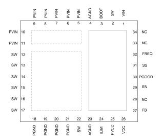
Figure 3. Pin Assignments, Bottom View
