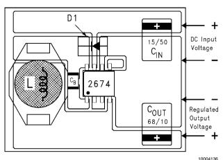
$$\begin{split} &C_{\text{IN}} - 15 \; \mu\text{F}, 25\text{V}, \text{Solid Tantalum Sprague, "594D series"} \\ &C_{\text{OUT}} - 68 \; \mu\text{F}, 10\text{V}, \text{Solid Tantalum Sprague, "594D series"} \\ &D1 - 1\text{A}, 40\text{V} \; \text{Schottky Rectifier}, \; \text{Surface Mount} \\ &L1 - 47 \; \mu\text{H}, \text{L13}, \; \text{Coilcraft DO3308} \end{split}$$
