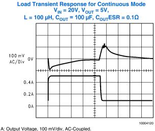
A: Output Voltage, 100 mV/div, AC-Coupled
