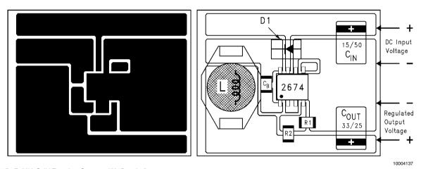
$C_{IN}$  - 15  $\mu F,$  50V, Solid Tantalum Sprague, "594D series"  $C_{OUT}$  - 33  $\mu F,$  25V, Solid Tantalum Sprague, "594D series"
