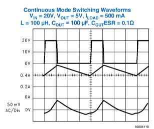
A: V<sub>SW</sub> Pin Voltage, 10 V/div.
