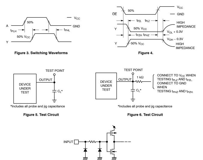
Figure 7. Input Equivalent Circuit
