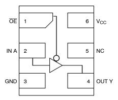
Figure 1. Pinout (Top View)
