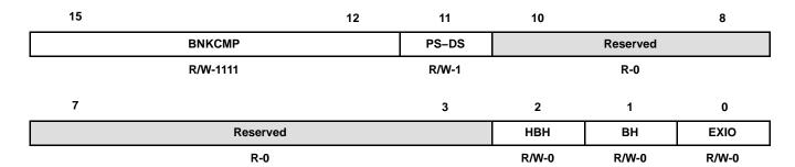
Figure 3–7. Bank-Switching Control Register (BSCR) [MMR Address 0029h]
