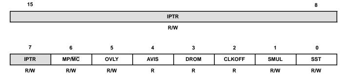
Figure 3-4. Processor Mode Status (PMST) Register
