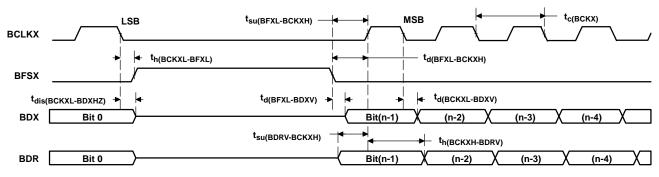
Figure 6-24. McBSP Timing as SPI Master or Slave: CLKSTP = 11b, CLKXP = 0
