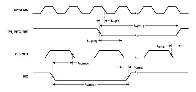
Figure 6–14. Reset and BIO Timings
