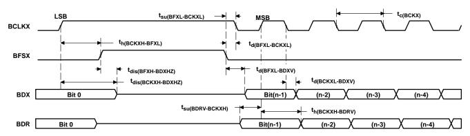
Figure 6-25. McBSP Timing as SPI Master or Slave: CLKSTP = 10b, CLKXP = 1
