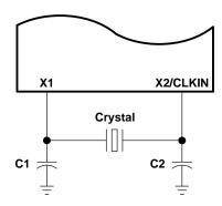
Figure 6-2. Internal Oscillator With External Crystal
