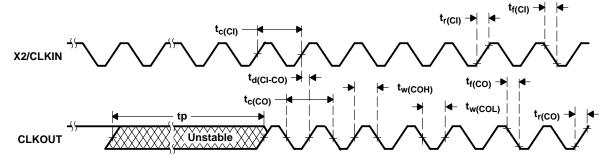
Figure 6-4. External Multiply-by-One Clock Timing
