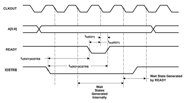
Figure 6-11. I/O Read With Externally Generated Wait States
