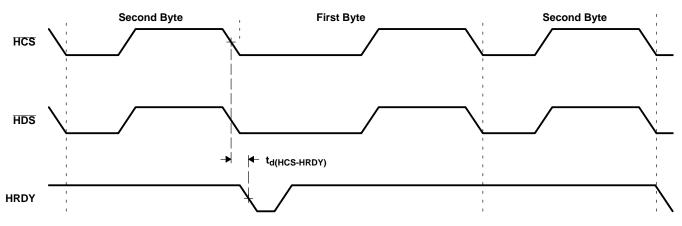
Figure 6-28. Using HCS to Control Accesses
