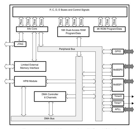
Figure 3–1. Block Diagram of the TMS320UC5405
