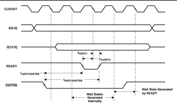
Figure 6-12. I/O Write With Externally Generated Wait States
