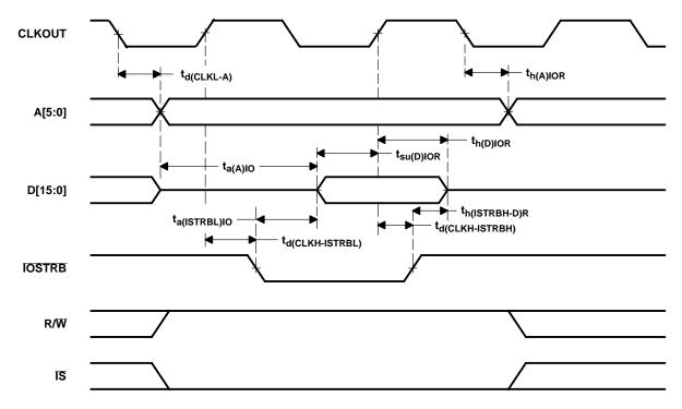
Figure 6-7. Parallel I/O Port Read
