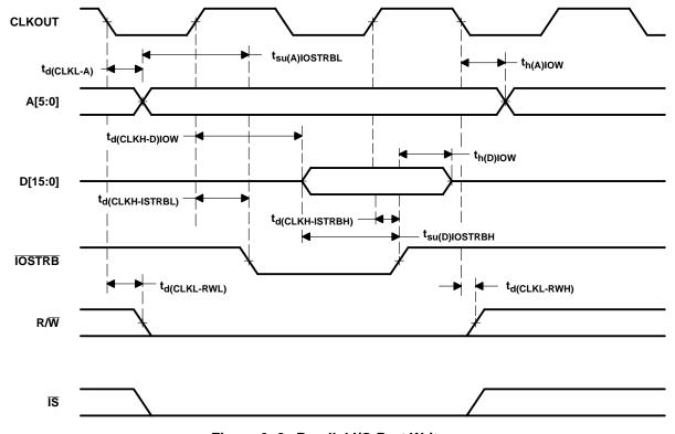
Figure 6-8. Parallel I/O Port Write
