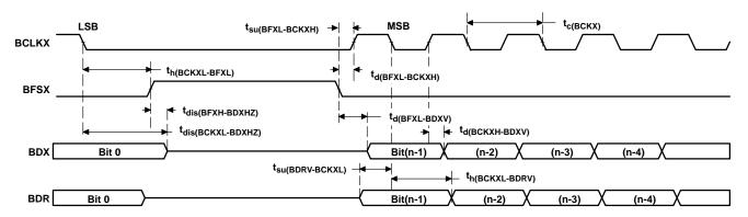
Figure 6-23. McBSP Timing as SPI Master or Slave: CLKSTP = 10b, CLKXP = 0
