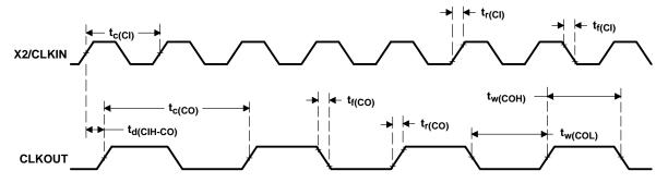
Figure 6-3. External Divide-by-Two Clock Timing
