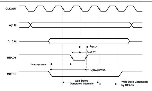
Figure 6-10. Memory Write With Externally Generated Wait States
