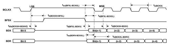
Figure 6-26. McBSP Timing as SPI Master or Slave: CLKSTP = 11b, CLKXP = 1
