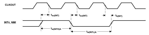
Figure 6–15. Interrupt Timing
