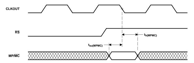
Figure 6–16. MP/MC Timing
