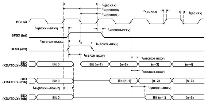
Figure 6-21. McBSP Transmit Timings
