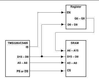
Figure 3-3. TMS320UC5405 External Memory Paging Scheme
