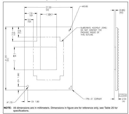
Figure 20. Surface-mount BGA2 Package - Top and Side View
