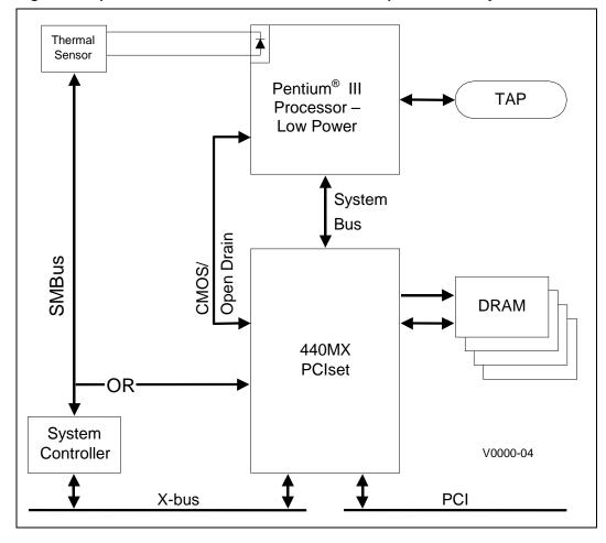
Figure 2. Signal Groups of a Pentium<sup>®</sup> III Processor/440MX Chipset - Based System
