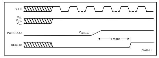
The PWRGOOD signal, which must be supplied to the processor, is used to protect internal circuits against voltage sequencing issues. The PWRGOOD signal should be driven high throughout boundary scan operation.
