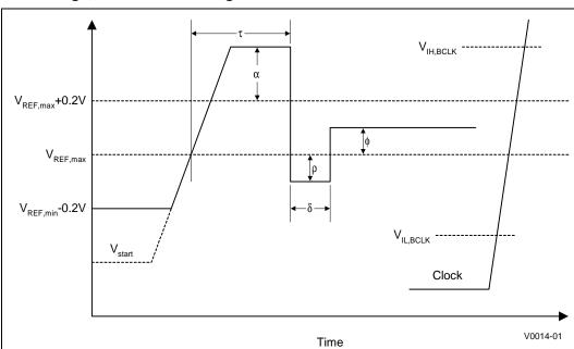
Figure 17. Low to High, GTL+ Receiver Ringback Tolerance
