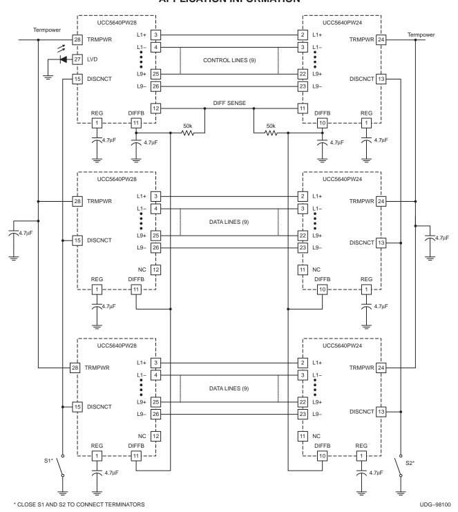
Figure 1. Application Diagram
