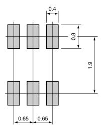
RemarkThe mounting pad layout in this document is for reference only.When designing PCB, please consider workability of mounting, solder joint reliability, prevention of solder<br/>bridge and so on, in order to optimize the design.
