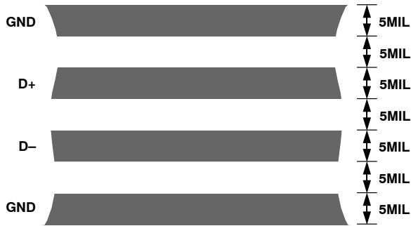
Figure 34. Typical Arrangement of Signal Tracks
