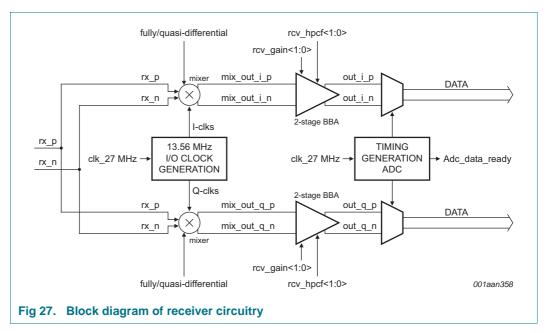
The receiver can also be operated in a single ended mode. In this case the Rcv\_RX\_single has to be set. In the single ended use case two receiver pins RXP and RXN need to be connected and will provide a single ended signal to the receiver circuitry.
