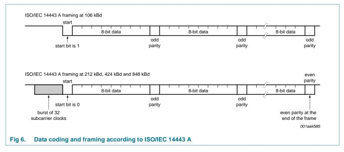
The internal CRC coprocessor calculates the CRC value based on ISO/IEC 14443 A part 3 and handles parity generation internally according to the transfer speed.
