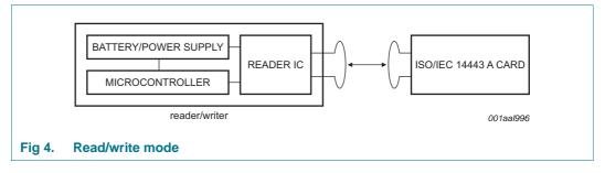
A typical system using the CLRC663 is using a microcontroller to implement the higher levels of the contactless communication protocol and a power supply (battery or external supply).
