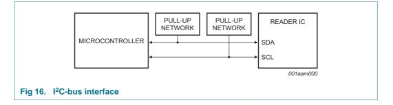
SDA is a bidirectional line, connected to a positive supply voltage via a pull-up resistor. Both lines SDA and SCL are set to HIGH level if no data is transmitted. Data on the I<sup>2</sup>C-bus can be transferred at data rates of up to 400 kbit/s in fast mode, up to 1 Mbit/s in the fast mode+.
