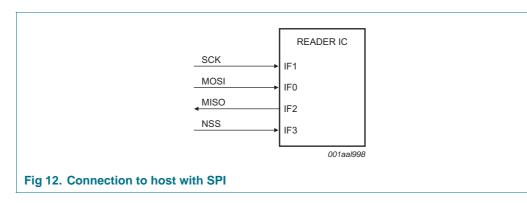
The CLRC663 acts as a slave during the SPI communication. The SPI clock SCK has to be generated by the master. Data communication from the master to the slave uses the Line MOSI. Line MISO is used to send data back from the CLRC663 to the master.
