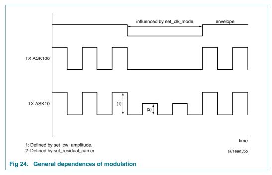
Note: When changing the continuous wave, the residual carrier also changes, while the modulation index remains the same.
