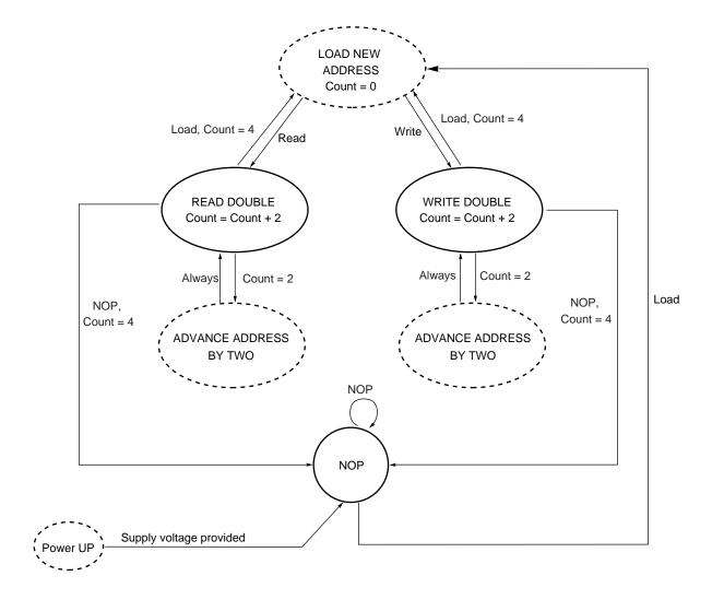
**Remarks 1.** A0 and A1 are internally advanced in accordance with the burst order table.
