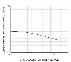
Figure 3.  $C_{RE}$ - $V_{CB}$
