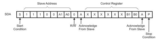
Figure 8. Write Control Register
