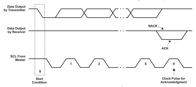
Figure 7. Acknowledgment on I<sup>2</sup>C Bus
