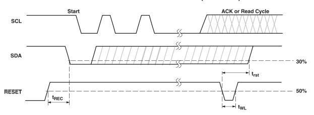
Figure 2. Reset Timing
