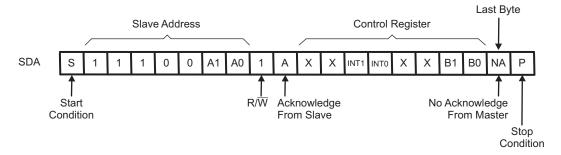
Figure 9. Read Control Register
