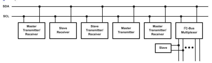
Figure 6. System Configuration
