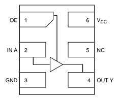
Figure 1. Pinout (Top View)
