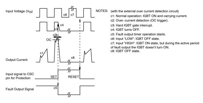
**Figure 7. Over Current Protection**
