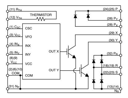
Figure 2. Internal Block Diagram
