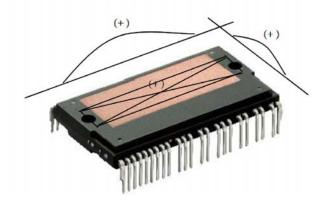
Figure 5. Flatness Measurement Position
