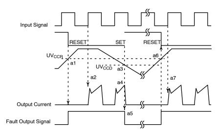
$NOTES: \ a1: Control \ supply \ voltage \ rises: \ after \ the \ voltage \ rises: \ UV_{CCR}, \ the \ circuits \ start \ to \ operate \ when \ the \ next \ input \ is \ applied.$
