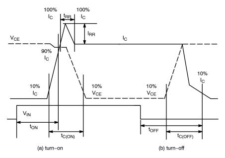
Figure 3. Switching Time Definition
