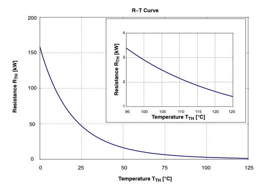
Figure 4. R-T Curve of the Built-in Thermistor
