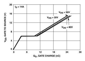
FIGURE 14. GATE TO SOURCE VOLTAGE vs GATE CHARGE
