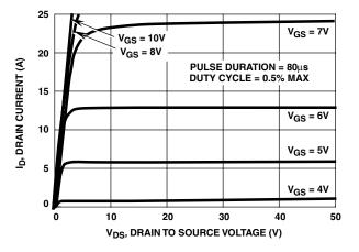
FIGURE 5. OUTPUT CHARACTERISTICS
