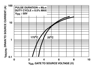
FIGURE 7. TRANSFER CHARACTERISTICS
