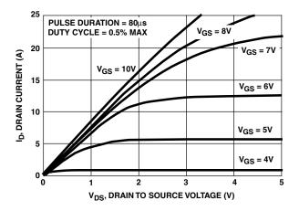
FIGURE 6. SATURATION CHARACTERISTICS
