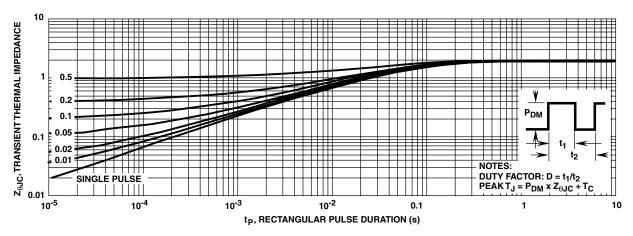
FIGURE 3. MAXIMUM TRANSIENT THERMAL IMPEDANCE
