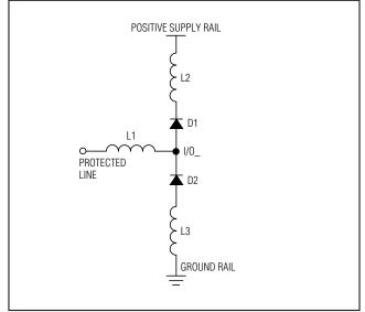
Figure 1. Parasitic Series Inductance
