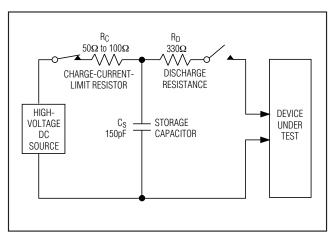
Figure 6. IEC 61000-4-2 ESD Test Model
