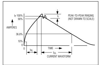
Figure 5. Human Body Model Current Waveform
