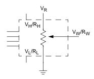
Three terminal potentiometer; variable voltage divider
