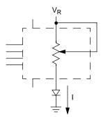
Two terminal variable resistor; variable current
