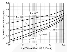
Figure 1. Forward Voltage vs. Forward Current
