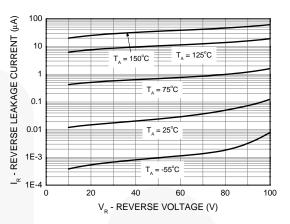
Figure 2. Reverse Voltage vs. Reverse Current
