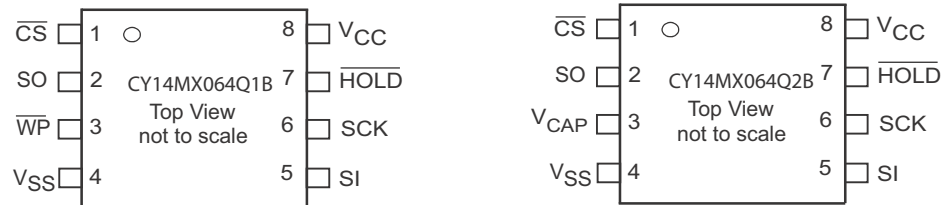
Figure 1. 8-pin SOIC pinout [1, 2]
