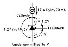
Figure 66. Voltage Associated with Reference (current source I<sub>r</sub> is external)
