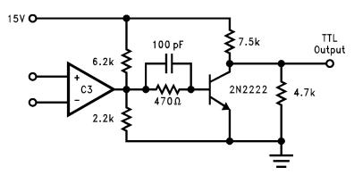
Figure 82. Wide-Input Range Comparator with TTL Output
