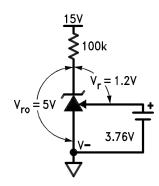
Figure 69. Thevenin Equivalent of Reference with 5V Output
