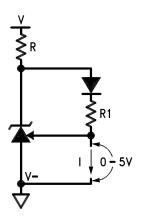
Figure 75. Proportional-to-Absolute-Temperature Current Source
