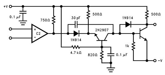
Figure 78. High Speed Level Shifter. Response Time is Approximately 1.5  $\mu$ s, Where Output is Either Approximately +V or -V.
