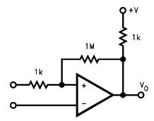
Figure 83. Comparator with Hysteresis ( $\Delta V_H = {}^+V(1k/1M)$ )
