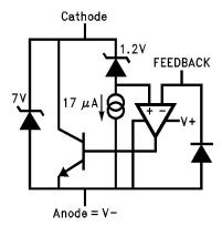
Figure 67. Reference Equivalent Circuit
