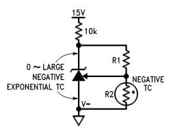
Figure 71. Output Voltage has Negative Temperature Coefficient (TC) if R2 has Negative TC
