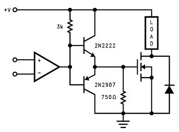
Figure 77. High Current, High Voltage Switch
