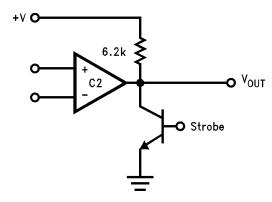
Figure 81. Basic Comparator with External Strobe
