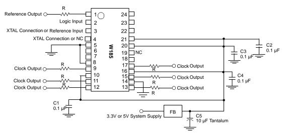
Figure 4. Recommended Circuit Configuration
