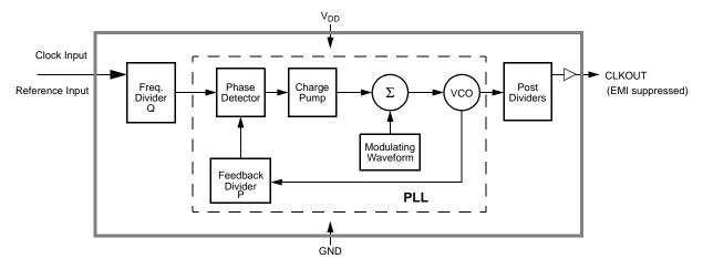
Figure 1. Functional Block Diagram
