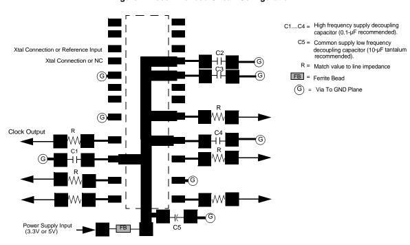
Figure 5. Recommended Board Layout (2-Layer Board)
