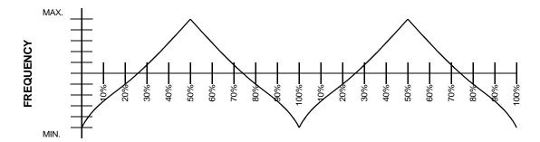
Figure 3. Typical Modulation Profile
