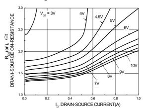
Figure 4. On-Resistance Variation with Gate-Source Voltage
