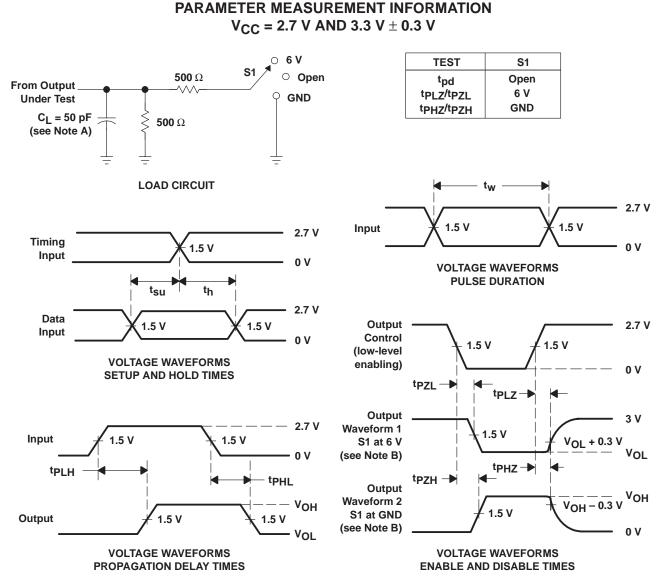
JOTES: A. CL includes probe and jig capacitance.
