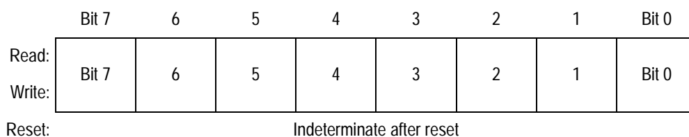
Figure 10-15. TIM Channel 1 Register Low (TCH1L)
