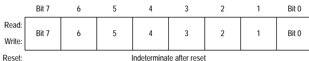
Figure 10-13. TIM Channel 0 Register Low (TCH0L)
