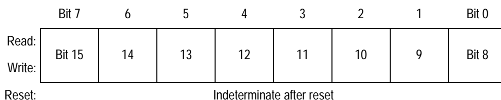
Figure 10-12. TIM Channel 0 Register High (TCH0H)
