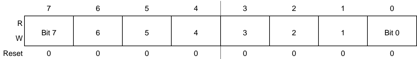
Figure 17-8. Timer x Counter Modulo Register Low (TPM1MODL)
