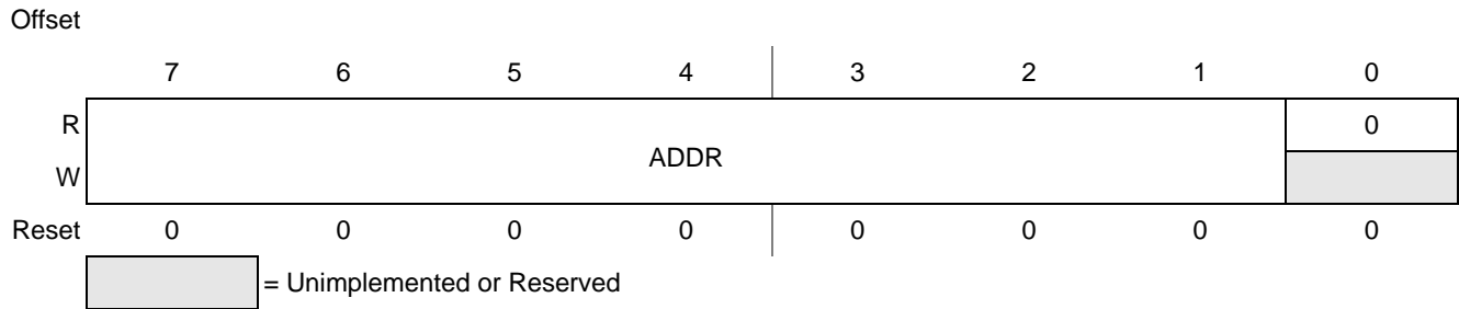
Figure 19-2. IIC Address Register (IIC1A)
