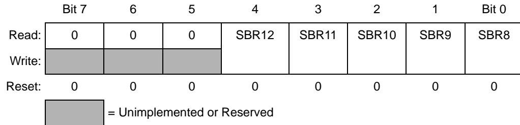
Figure 18-4. SCI1 Baud Rate Register (SCIxBDH)
