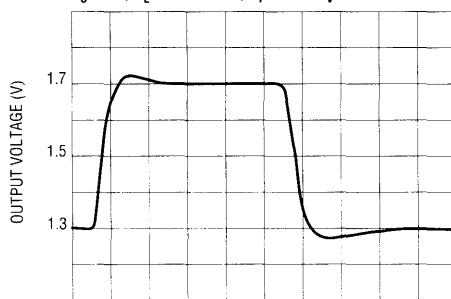
Small Signal Pulse Response (Single Supply) V_S = +5V , R_L = 150\Omega to OV , R_F = 1K\Omega , A_V = +2
