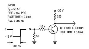
Figure 1. Delay and Rise Time Test Circuit
