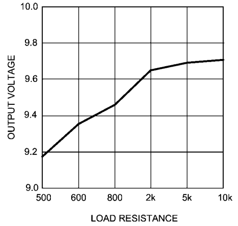
Output Voltage vs Load Resistance V_{DD} = 15V , V_{SS} = -15V , THD+N = 0.1%
