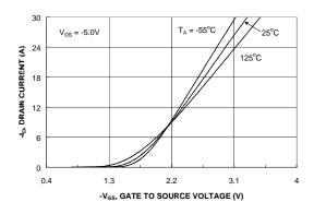
Figure 5. Transfer Characteristics.
