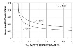
Figure 4. On-Resistance Variation with Gate-to-Source Voltage.
