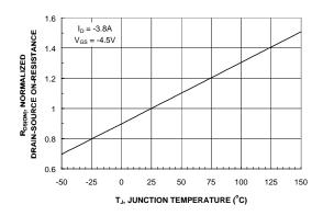
Figure 3. On-Resistance Variation with Temperature.
