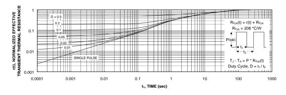
Figure 11. Transient Thermal Response Curve.
