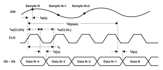
Figure 1. Timing Diagram
