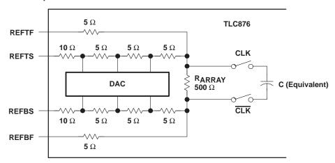
Figure 17. TLC876 Equivalent Reference Structure
