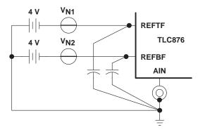
Figure 22. Recommended Bypassing For The Reference
