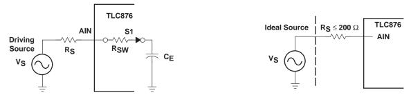
Figure 12. TLC876 Simplified Equivalent Input
