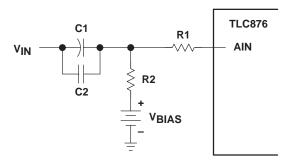
Figure 14. AC-Coupled Inputs
