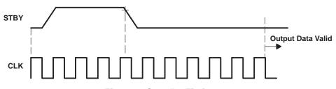
Figure 3. Standby Timing
