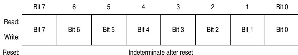
Figure 3-5. ADC Data Register (ADR)
