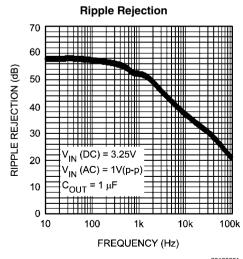
70 60 RIPPLE REJECTION (dB) 50 40 30 V<sub>IN</sub> (DC) = 3.25V 20  $V_{|N}(AC) = 1V(p-p)$ 10 o t 10 10k 100k 1k FREQUENCY (Hz) 20126819
