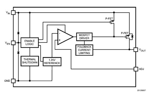
FIGURE 2. LP38693-ADJ Functional Diagram (SOT-223, LLP)
