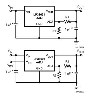
$V_{OLIT} = V_{AD.1} x (1 + R1/R2)$
