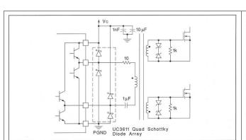
Figure 5. Transformer Coupled Push-Pull MOSFET Drive
