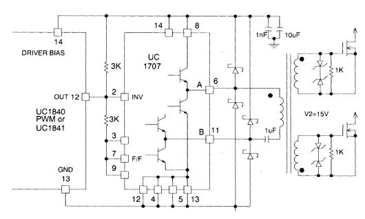
Figure 14. Convert Single Output PWMS High-Current Push-Pull Configuration
