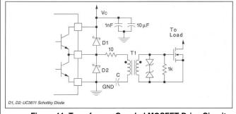
Figure 11. Transformer Coupled MOSFET Drive Circuit
