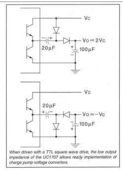
Figure 9. Charge Pump Circuits
