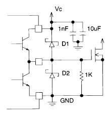
Figure 13. Power MOSFET Drive Circuit
