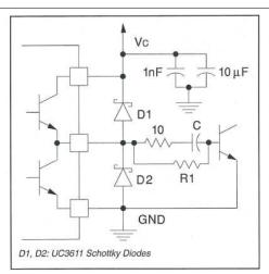
Figure 10. Power Bipolar Drive Circuit
