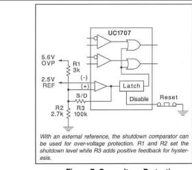
Figure 7. Overvoltage Protection
