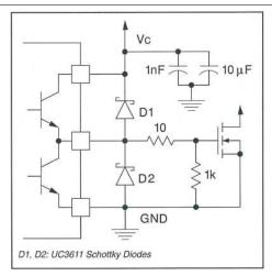
Figure 8. Power MOSFET Drive Circuit
