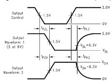
Waveform 1 is for an output with internal conditions such that the output is low except when disabled by the output control. Waveform 2 is for an output with internal conditions such that the output is HIGH except when disabled by the output control. All input pulses have the following characteristics: frequency = 10 MHz,  $t_r = t_f = 2$  ns,  $Z_O = 50\Omega$ . The outputs are measured one at a time with one transition per measurement.
