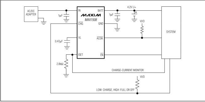
Figure 3. µP-Interfaced Li+ Battery Charger
