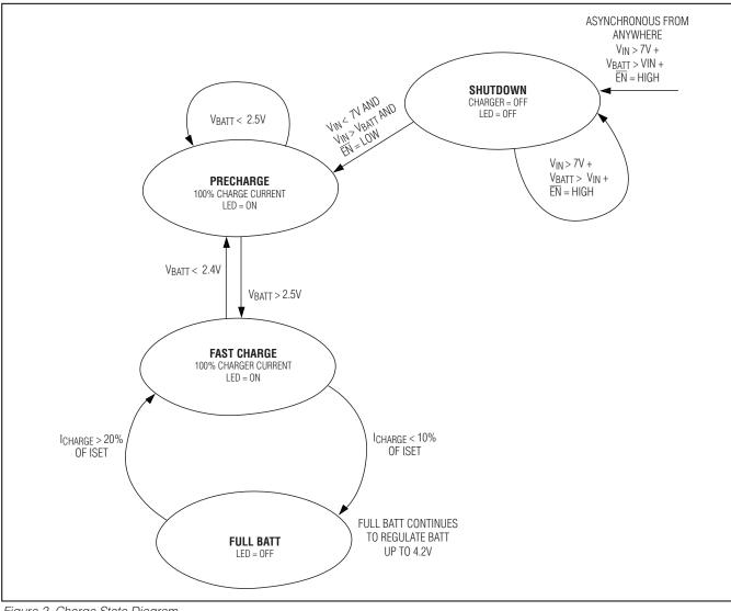
Figure 2. Charge State Diagram
