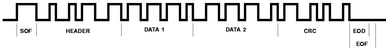
FIGURE 3. TYPICAL J1850 VPW MESSAGE FRAME
